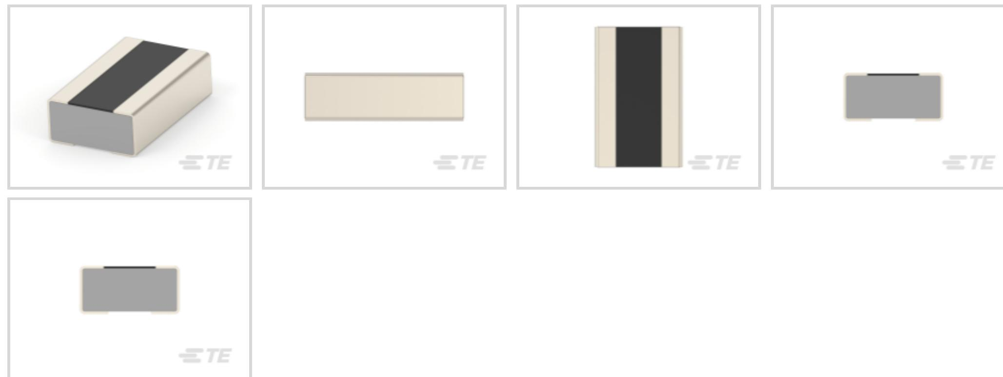
Resistor Type: **Current Sensing Resistor**Element Type: **Thick Film**Package Size Code: **0508**Power Rating: **1 W**Resistance Value: **.27  $\Omega$**
