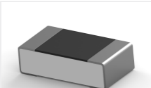
TE Part #8-2176370-8 RQ 0603 3K48 0.1% 10PPM 5K RL
