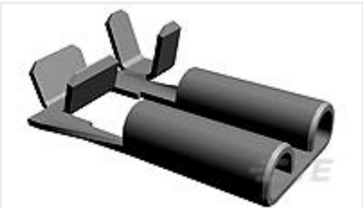
TE Part #1742086-2 187 FASTON,FLAG,REC.,18-22 AWG, TPBR
