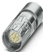
M23, Cable connector, series: M23 PRO, straight, shielded: yes, ONECLICK fast locking system, No. of pos.: 8+1, Direction of rotation: Standard, contact connection type: Pin, Crimp connection, cable diameter range: 6 mm ... 10 mm, coding: N, Item is lead-free in accordance with RoHS II without Exemption 6c (Pb < 0.1 %)
