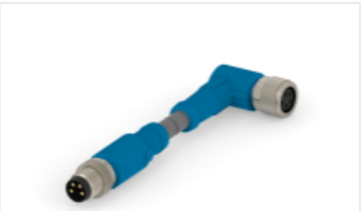
TE Part #T4062124004-005 RPC-M8-4MS-5.0SH-M8-4FR-PUR
