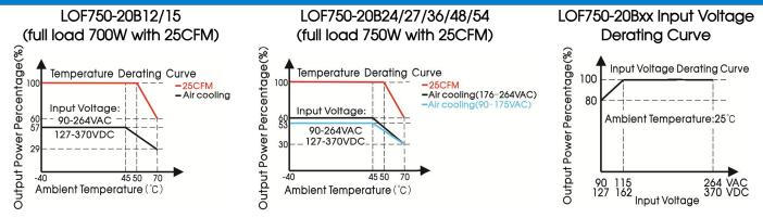
Note: With an AC input voltage between 90 - 115VAC and a DC input between 127 - 162VDC the output power must be derated as per the temperature derating curves.
