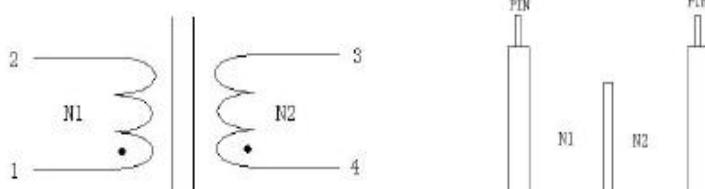
绕线结构表 Winding Structure Diagram
