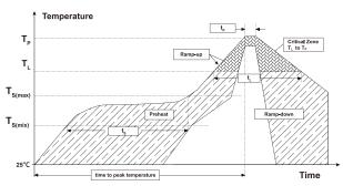
—All temperature refer to topside of the package, measured on the package body surface.
