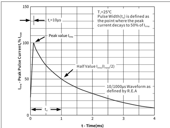
Fig. 3 Pulse Waveform
