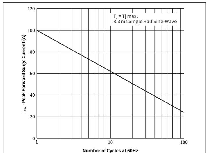
Fig. 6 Maximum Non-Repetitive Forward Surge Current Uni-Directional Only
