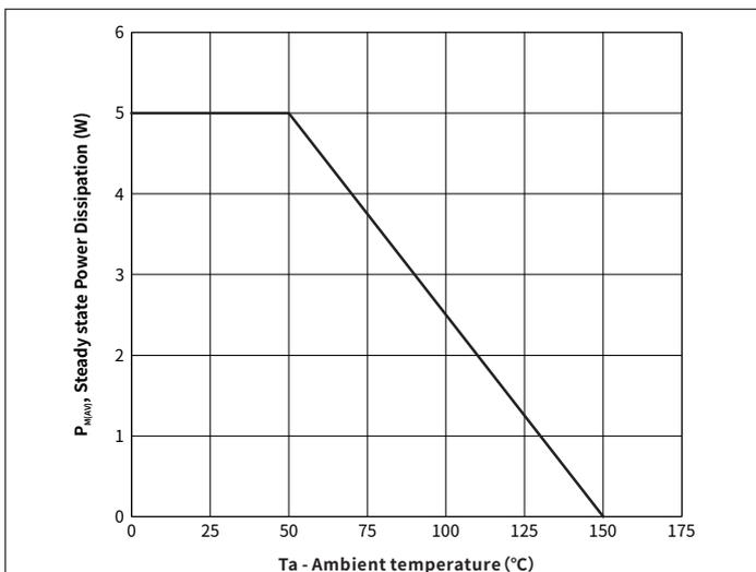
Fig. 5 Steady State Power Dissipation Derating Curve
