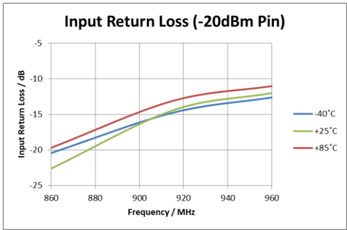
Figure 14: Input Return Loss (-20 dBm Pin)
