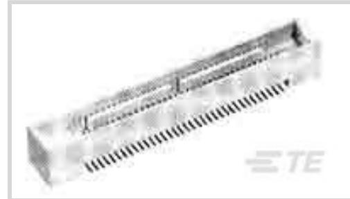
PCB Connector Assembly Type: **PCB Mount Header**PCB Mount Orientation: **Vertical**Connector System: **Board-to-Board**Number of Positions: **70**Number of Rows: **2**
