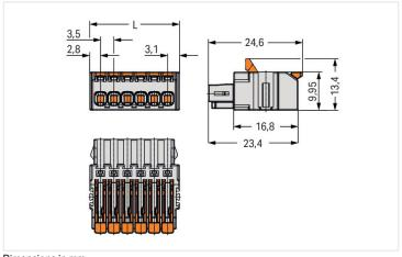
Dimensions in mm L = (pole no. x pin spacing) + 2.4 mm
