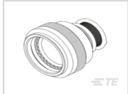
Connector Backshell Product Style: **Ruggedized**Connector Backshell Product Type: **Backshell**Cable Entry Diameter: **.2 – 19.1 mm [.01 – .75 in]**Primary Product Material: **Nickel Aluminum Bronze**Body Orientation: **Straight**
