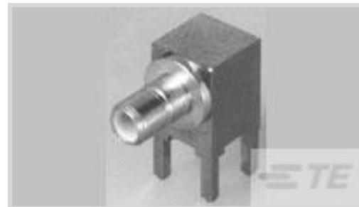
RF Interface: **SMB**RF Connector Style: **Jack**RF Connector Mated Outer Diameter (Approximate): **4.75 mm [ .187 in ]**Impedance: **50 Ω**RF Connector Coupling Mechanism: **Snap-On****All SMB Connector: Jack, Right-Angle Mount, Mated Outer Dia. 4.75mm (6)**
