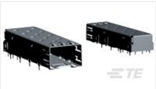
TE Part #2227023-1 CAGE ASSY PRESS FIT, SFP
