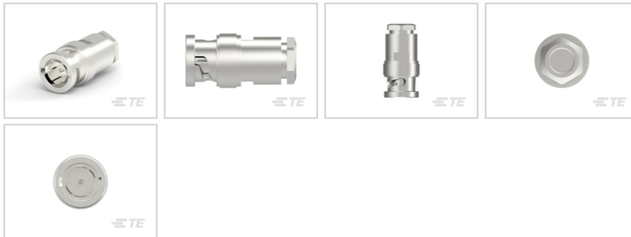
RF Interface: **BNC**RF Connector Style: **Plug**RF Connector Mated Outer Diameter (Approximate): **14.53 mm [ .572 in ]**Impedance: **75 Ω**Compatible With RF Cable Type: **PSF 1/3M, Raychem 9524A1311, Raychem 9524A1811, RG 140, RG 210, RG 59B, URM 90**
