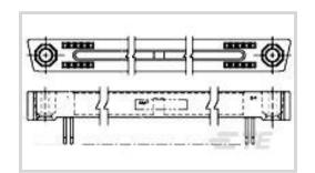
PCB Connector Assembly Type: PCB Mount Receptacle
