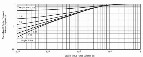
Normalized Thermal Transient Impedance, Junction-to-Foot
