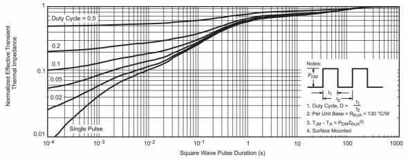
Normalized Thermal Transient Impedance, Junction-to-Ambient
