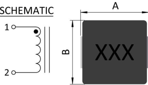
Shape and Dimensions(dimensions are in mm):
