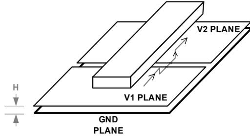
Figure 4-5 shows the thermal ground plane in relation to the return-path capacitor.
