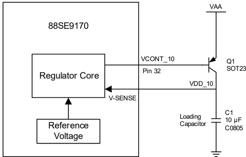
The BJT's supply voltage, **VAA**, can use the same source as the 88SE9170's **VAA1** or **VAA2**. The BJT and the internal regulator core forms a closed feedback loop to provide a stable voltage for **VDD\_10**.
