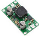
Pololu Adjustable 4-12V Step- Up/Step-Down Voltage Regulator S18V20ALV
