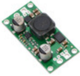
Pololu 5V Step- Up/Step-Down Voltage Regulator S18V20F5
