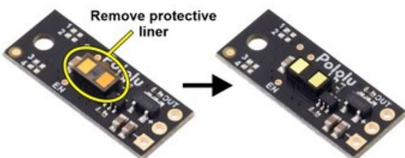
**Important note:** This product might ship with a protective liner covering the sensor IC. The liner must be removed for proper sensing performance.
