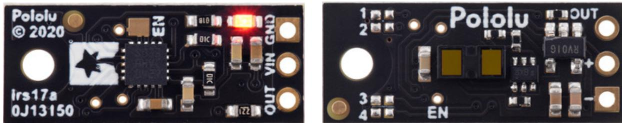
The board has an optional ENABLE pin that can be driven low to put it into a low-power state that consumes approximately 0.4 mA. This pin can be accessed through a via or its neighboring surface-mount pad on the back side labeled "EN" on the silkscreen. The ENABLE pin is pulled up to VIN, enabling the sensor by default.
