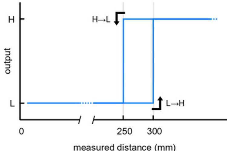
Please note that this sensor will only tell you *if* there is an object within the detection range along its line of sight, not how far away it is. As shown in the diagram above, there is hysteresis at the maximum range threshold to
