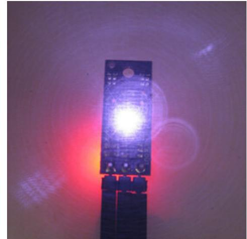
**A camera with no IR filter shows the infrared light emitted by a Pololu Digital Distance Sensor.**
