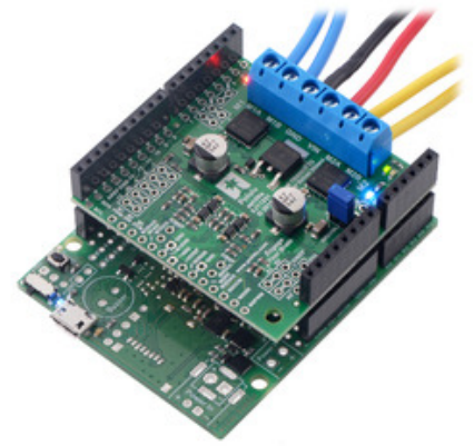
Dual TB9051FTG Motor Driver Shield for Arduino being controlled by an A-Star 32U4 Prime SV.
