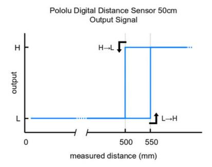
Please note that this sensor will only tell you if there is an object within the detection range along its line of sight, not how far away it is. As shown in the diagram above, there is hysteresis at the maximum range threshold to
