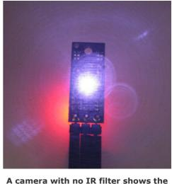
A camera with no IR filter shows the infrared light emitted by a Pololu Digital Distance Sensor.
