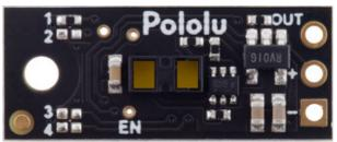
The board has an optional ENABLE pin that can be driven low to put it into a low-power state that consumes approximately 0.4 mA. This pin can be accessed through a via or its neighboring surface-mount pad on the back side labeled "EN" on the silkscreen. The ENABLE pin is pulled up to VIN, enabling the sensor by default.
