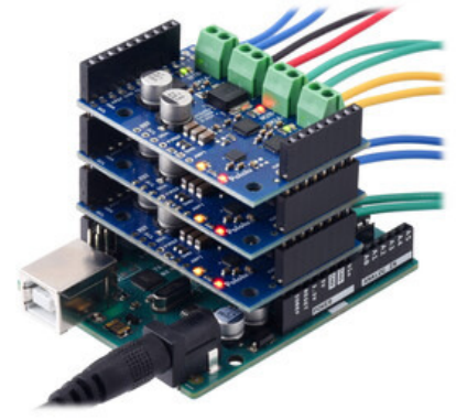
Three Motoron M3S256 shields being controlled by an Arduino Uno.
