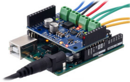
Motoron M3S256 shield being controlled by an Arduino Uno.
