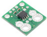
ACS724LLCTR-20AB Current Sensor Carrier -20A to +20A
