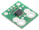
ACS724LLCTR-05AB Current Sensor Carrier -5A to +5A
