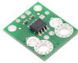
ACS724LLCTR-10AU Current Sensor Carrier 0A to 10A
