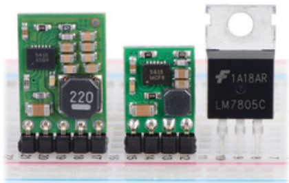
Pololu step-down voltage regulators D24V10Fx and D24V5Fx next to a 7805 voltage regulator in TO-220 package.
