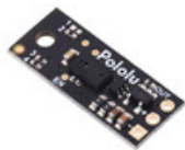
Pololu Distance Sensor with Pulse Width Output, 50cm Max
