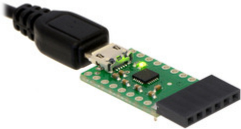
CP2104 USB-to-serial adapter carrier with included 6-pin 0.1” right-angle female header installed.
