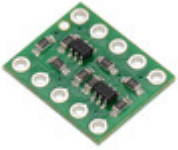
Logic Level Shifter, 4-Channel, Bidirectional
