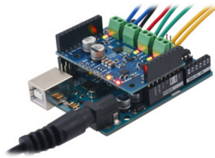
Motoron M3S550 shield being controlled by an Arduino Uno.
