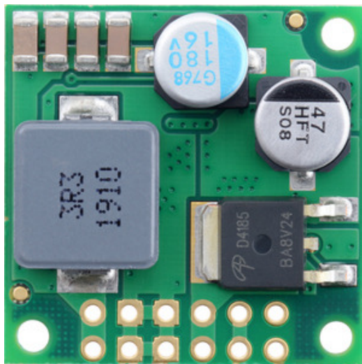
9V, 5A Step-Down Voltage Regulator D36V50F9, top view.
