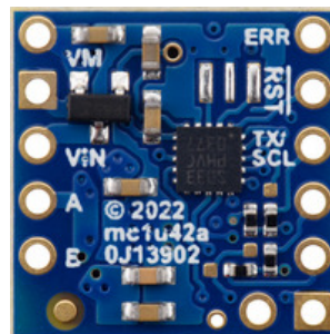
Motoron M1T256 Single I 2 C Motor Controller, bottom view.
