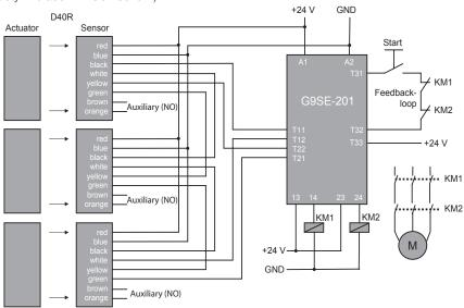
NOTE: For automatic reset connect the feedback loop between T31 and T33. Connect T32 to +24 VDC.
