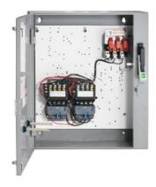
2-speed 3-phase motor starter Size 1 3/4 One winding consequent pole Constant or variable torque Solid-state overload relay High SPD OLR amp range 10-40A Low SPD OLR amp range 5.5-22A 110VAC 50HZ / 120VAC 60HZ coil Combination type 60Amp disconnect switch Enclosure NEMA type 4/12 Water/dust tight weather proof
