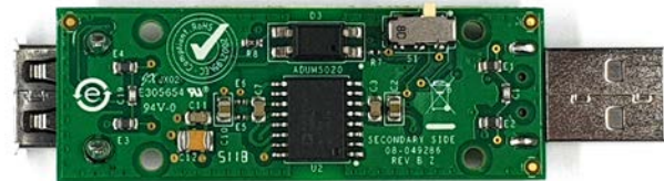
Figure 3. S1 Switch Position for Full Speed Operation
