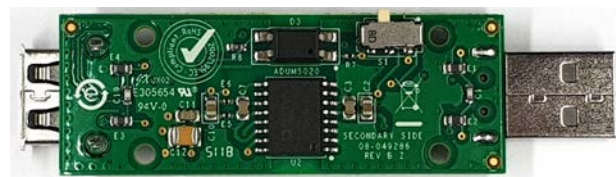
Figure 4. S1 Switch Position for Low Speed Operation
