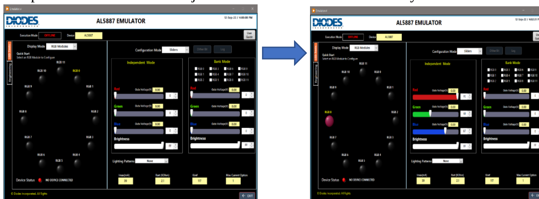
Figure 25: Configuring LEDs in RGB Modules & Independent Mode
