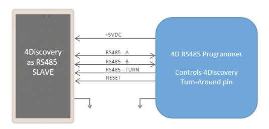
This is the situation used when programming the 4Discovery using the 4D RS485 Programmer.
