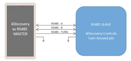
This image shows the 4Discovery when acting as Master, connecting to a Slaved device that is incapable of Auto turn-around but can have its RS485 chip controlled externally by the 4Discovery. Not a typical situation.
