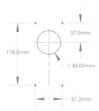
The 4 corner holes are slots on the plastic, which give some tolerance when mounting. The slots allow for 51.15mm to 56.15mm horizontal centres.
