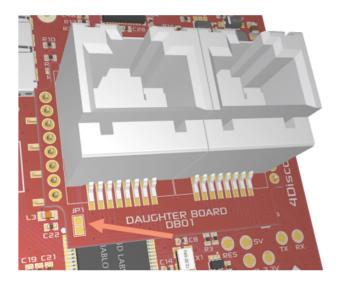
Arrow pointing to the JP1 pads which are used to enable the 120 $\Omega$  Termination Resistor for RS485
