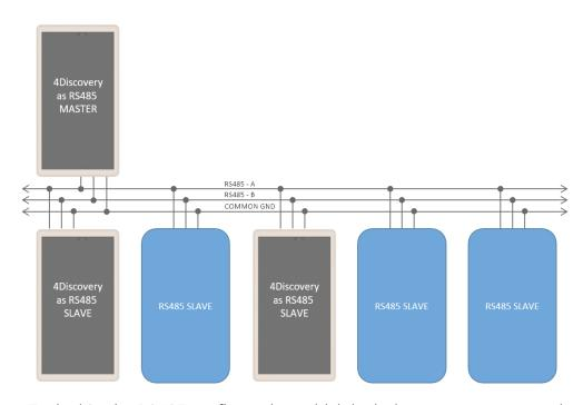
Typical 2-wire RS485 configuration, which includes a common ground
