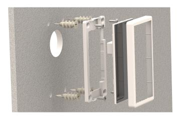
As illustrated above, the wall is on the left, which shows the recommended drill holes for the module.
