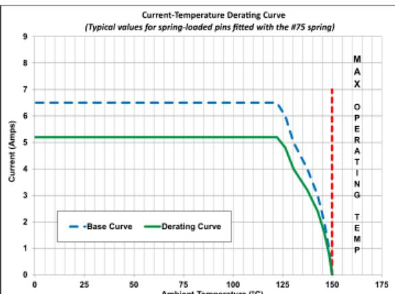
The stroke, force and current rating values are measured using spring pins with an internal construction per the design specification. Individual spring pin performance may vary from these values based on design differences.
