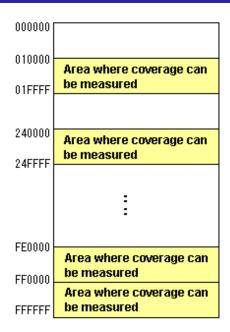
Figure 5.107 Schematic of Data Coverage Memory Allocation
