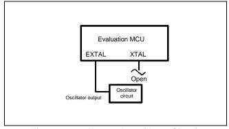
Figure 2.8 External Oscillator Circuit
