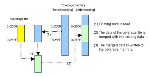
Figure 5.102 Schematic of the Merge Mode
