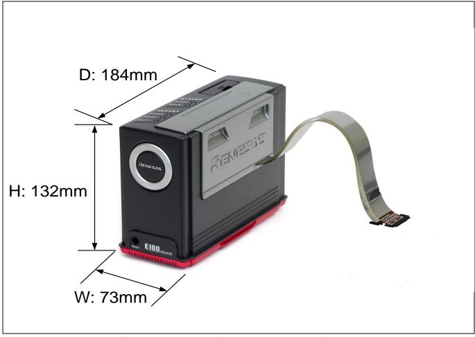
Figure 7.2 External Dimensions of the E100 Emulator
