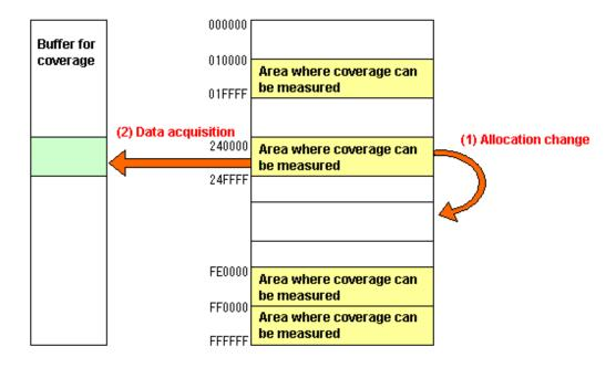
Figure 5.108 Schematic of Data Coverage Memory Allocation Change
