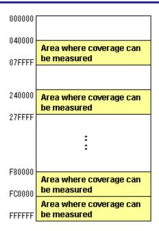
Figure 5.76 Schematic of Coverage Memory Allocation
