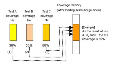
Figure 5.103 Schematic of Merge-Mode Application
