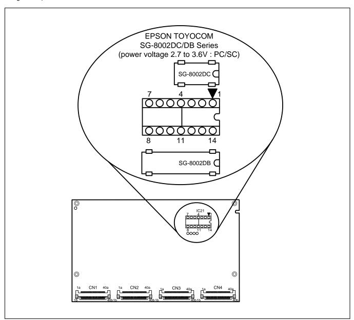
Figure 2.7 Replacing the Oscillator Module
