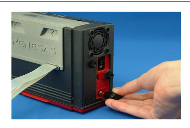
Figure 2.5 Connecting the Emulator Power Supply
