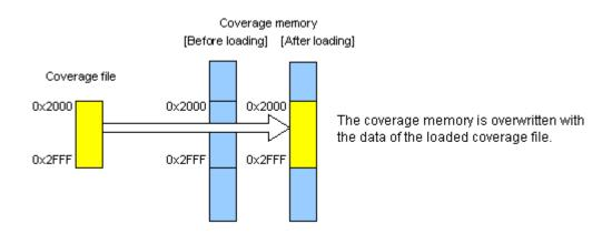
Figure 5.101 Schematic of the Overwrite Mode
