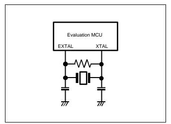
Figure 2.9 Circuit in which Oscillation does not Occur
