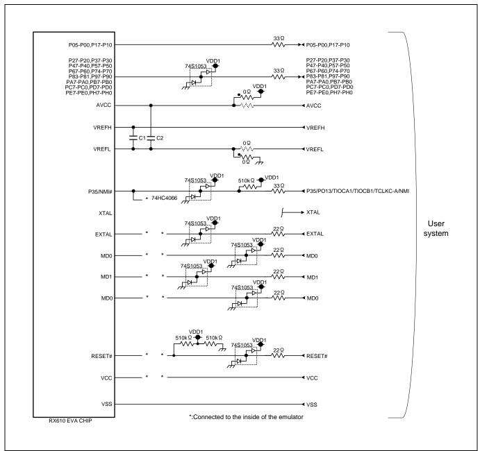
Figure 7.1 Connection Diagram for R0E556100MCU00 (Partial)
