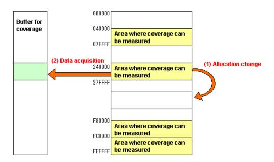
Figure 5.77 Schematic of Coverage Memory Allocation Change
