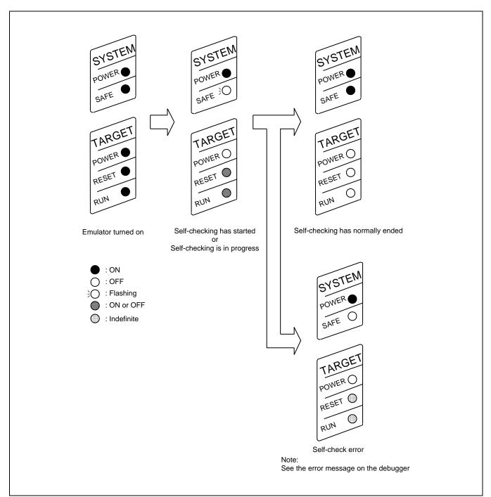
Figure 2.6 LED Displays during the Self-Checking
