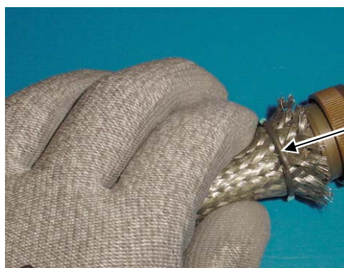
Figure 3. Raychem Side Entry Tinel-Lock Ring Latched in Place
