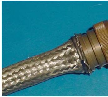
Figure 5. Trimming the Excess Braid
