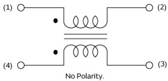
Note1: The Port/Pin No. of the Simulation Model provided by our company is as follows.
