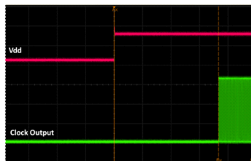
Figure 16. Startup Waveform vs. Vdd
