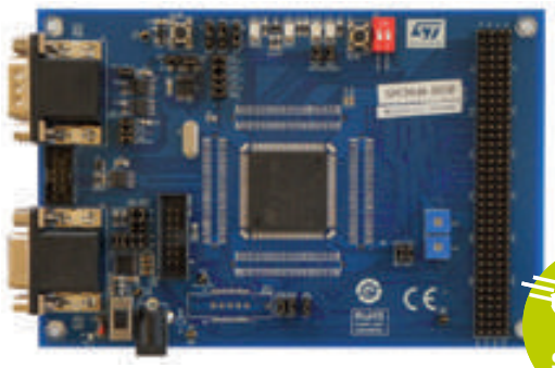
Discovery Kit for the A Line with SPC564A70L7. order code: SPC564A-DISP
