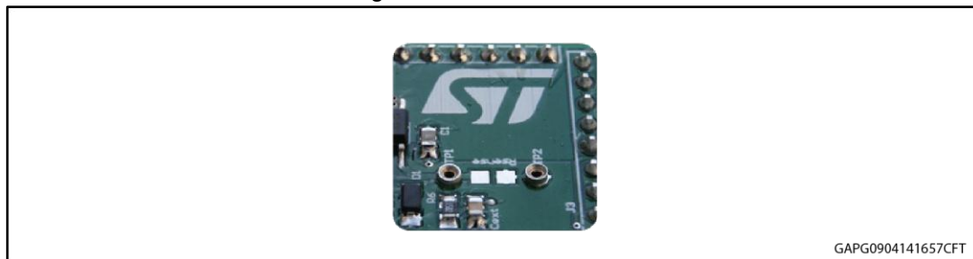
Figure 4: Mounting through-hole sense resistor
