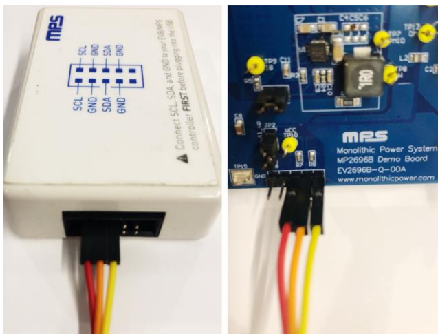
Figure 5: EVB to MPS I 2 C Communication Interface Wire Connection
