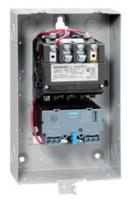
Non-reversing motor starter Size 1 Single phase full voltage Solid-state overload relay OLRelay amp range 0.75-3.4A 190-220/220-240V 50/60HZ coil Combination type Indoor general purpose use
