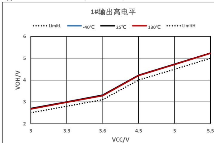
Figure 7-7 Receiver Output @ Logic-high
