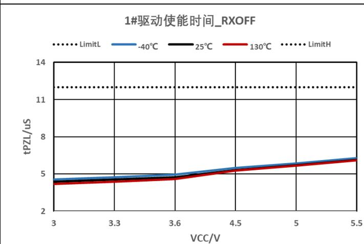
Figure 7-12 Driver Enable Time vs. Supply Voltage:  $t_{PZL}$
