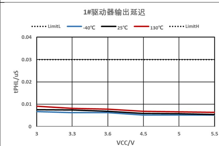
Figure 7-10 Driver Propagation Delay vs. Supply Voltage (H to L)
