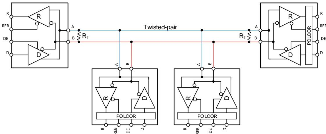
Figure 10-1. Typical RS-485 Network With CS485 Half-Duplex Transceivers
