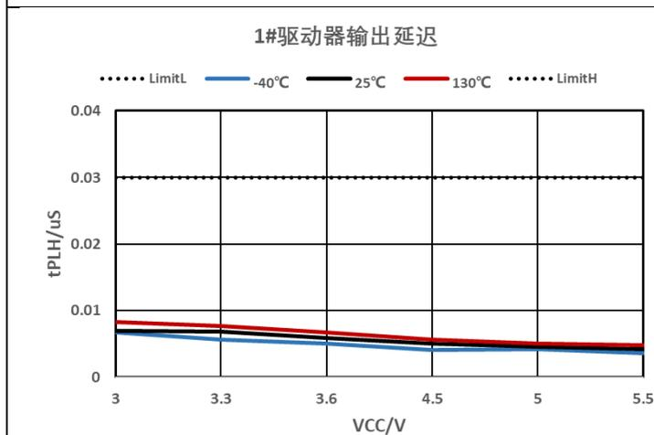
Figure 7-9 Driver Propagation Delay vs. Supply Voltage (L to H)
