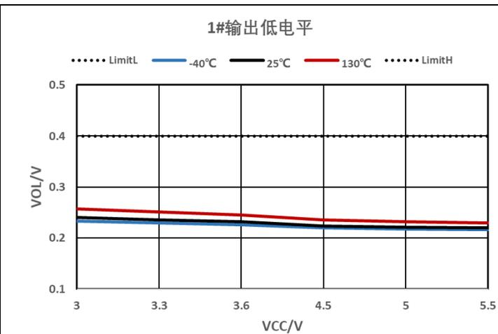
Figure 7-8 Receiver Output @ Logic-low
