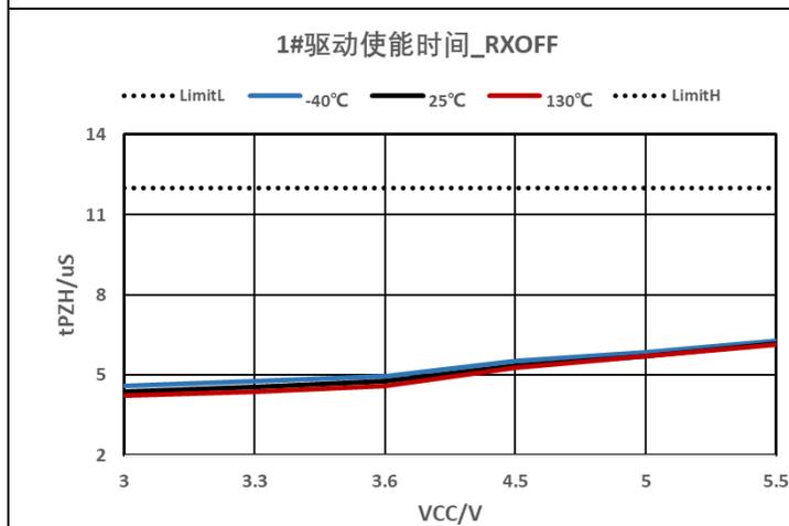
Figure 7-11 Driver Enable Time vs. Supply Voltage:  $t_{PZH}$
