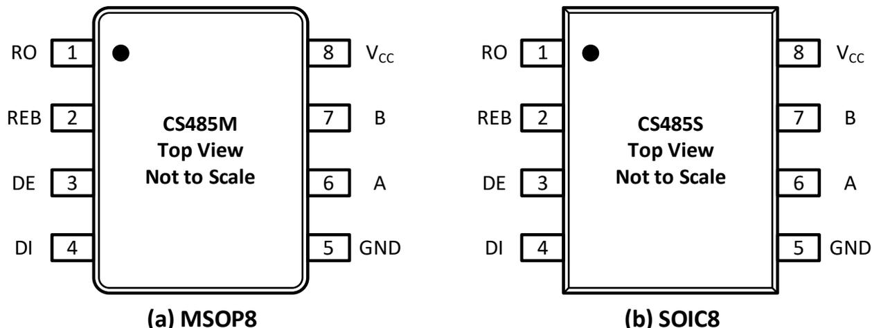
**Figure 6-1. CS485 pin configuration**
