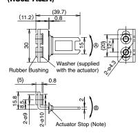
The mounting center distance is set to 12 mm at factory. When 20-mm distance is required, adjust the distance by moving the rubber bushings.
