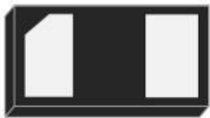
DFN1006-2L (Bottom View)
