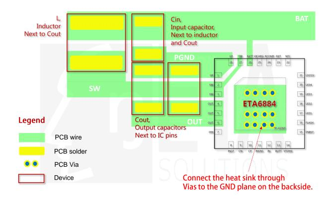
Please try to place the Cout, L, and Cin as suggested by the illustration above. The Cout has to be placed just next to the chip with shortest wire to the OUT and PGND pins. And SW wire goes underneath the Cout and connected by a power inductor just next to the Cout. With the Cin placed beside, a very tight and small power loop is achieved to improve EMI characteristic.
